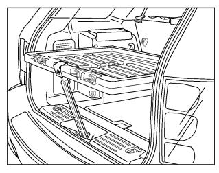
Your vehicle has an adjustable panel that also functions as a table. The maximum load for the table is 100 lbs. distributed (45 kg).
